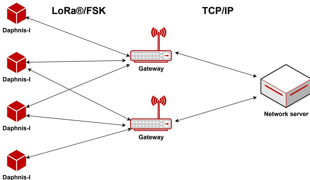
Figure 29: LoRaWAN® network setup
