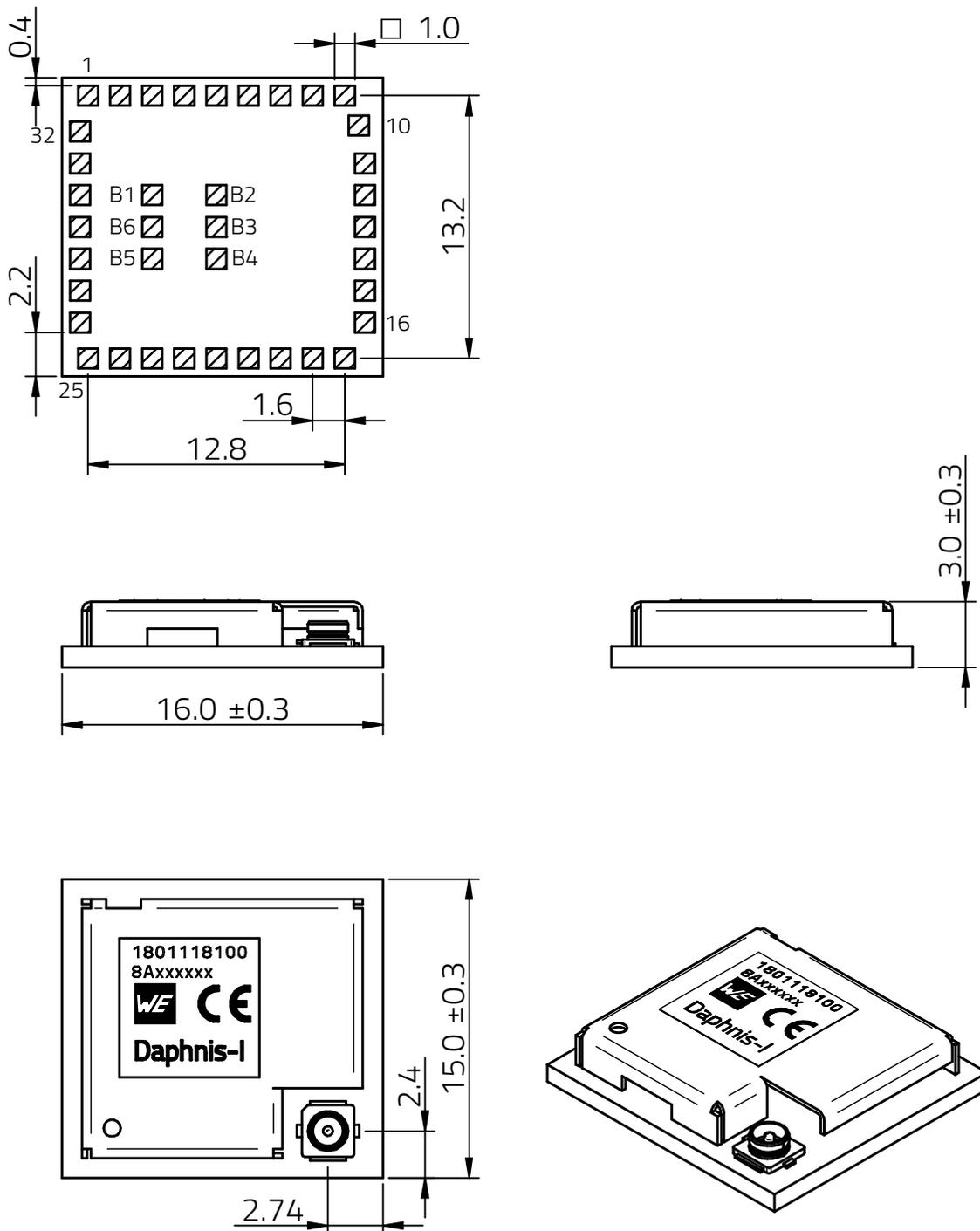
Figure 54: Module dimensions [mm]
