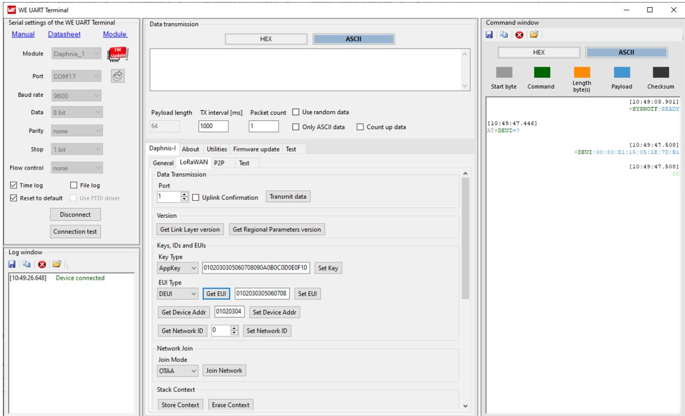
Figure 11: WE UART Terminal AT+DEUI command
