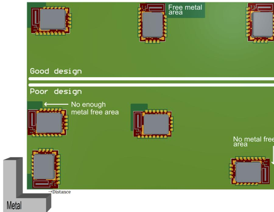
Figure 45: Placement of the module with integrated antenna
