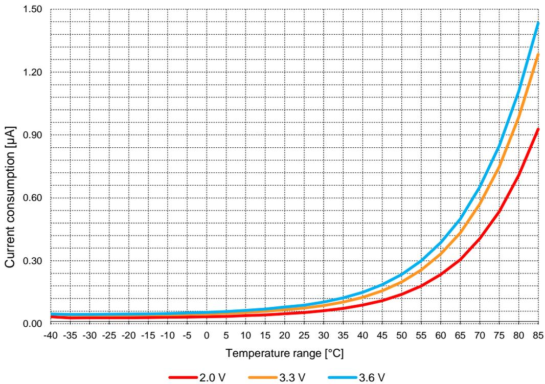
Figure 3: Current consumption during Sleep mode
