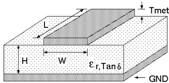
Figure 46: Dimensioning the antenna connection as micro strip
