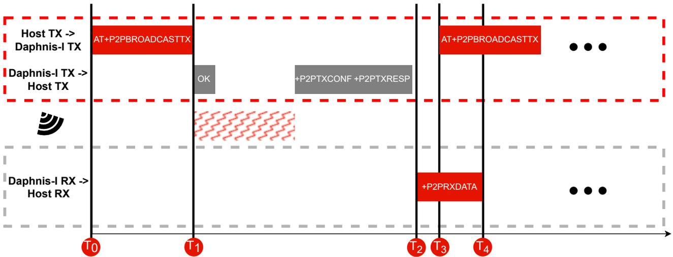
Figure 40: Command sequence when transmitting data
