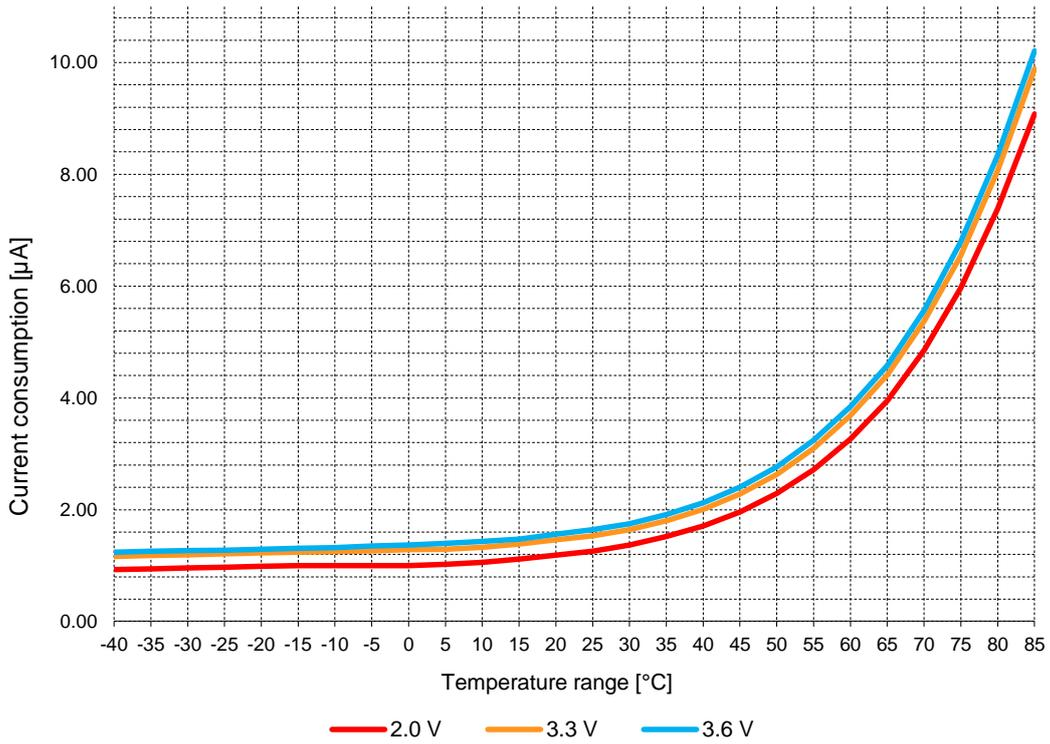
Figure 4: Current consumption during Idle state
