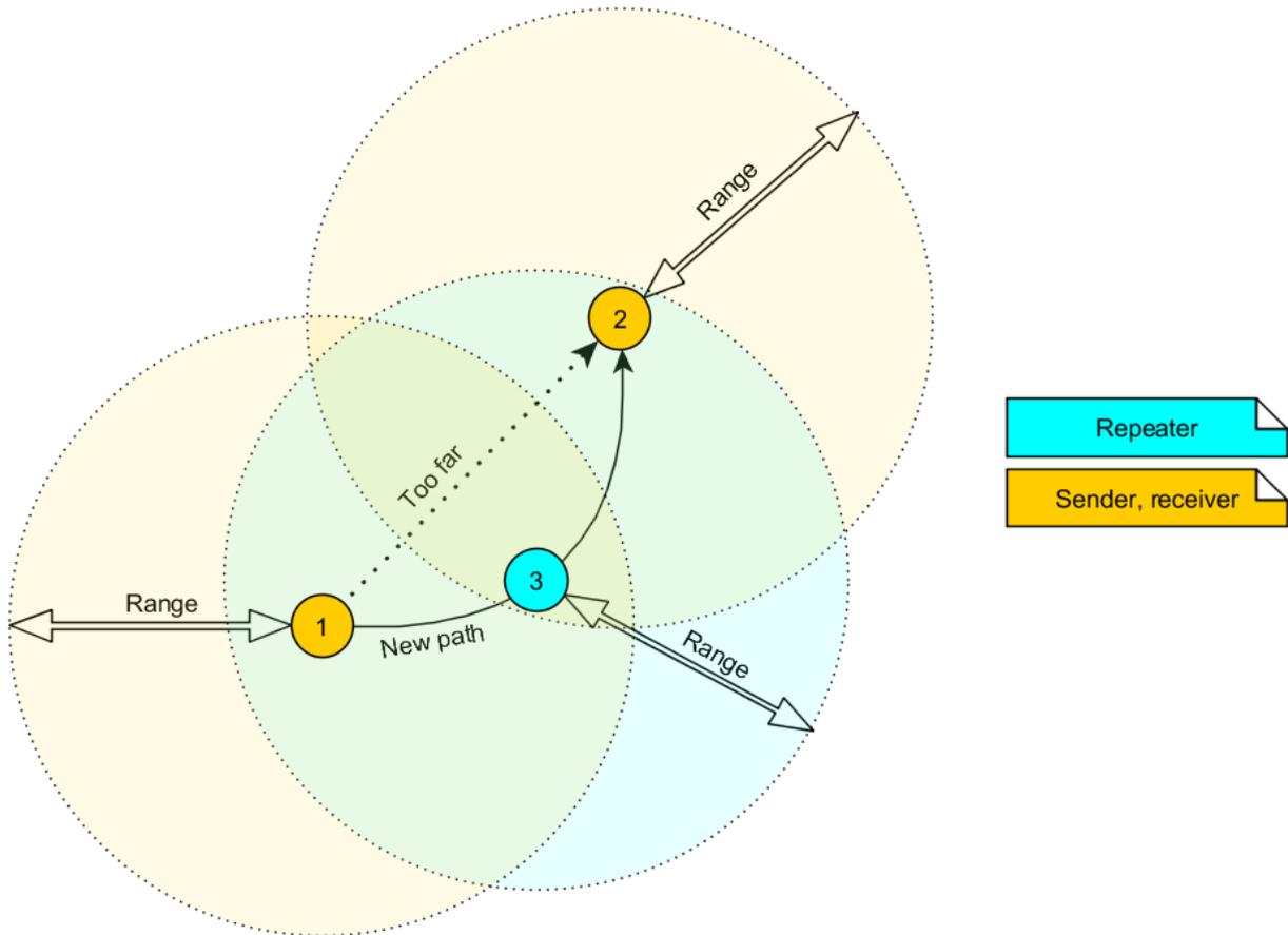
Figure 34: Range extension using several repeaters
