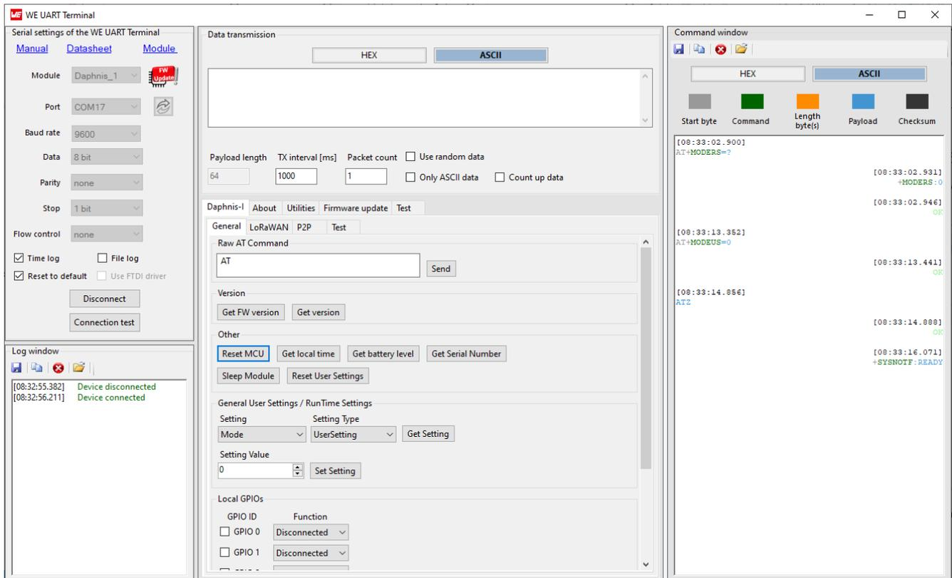
Figure 10: WE UART Terminal switch to LoRaWAN® MODE
