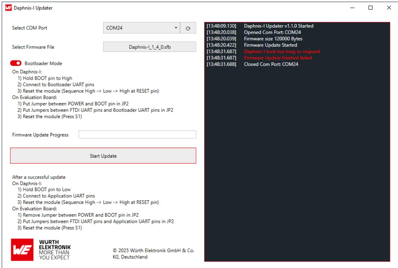
Figure 43: Daphnis-I Updater failure
