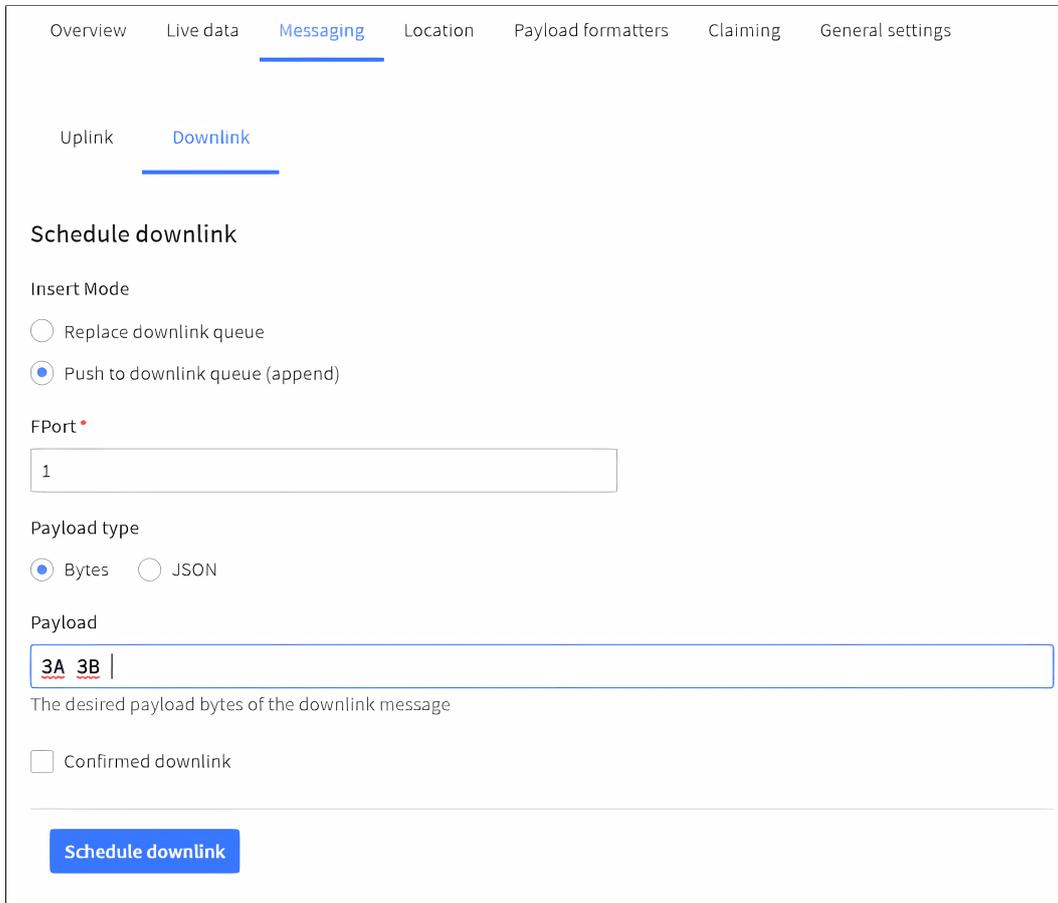
The screenshot shows the TTN console interface for scheduling a downlink. The 'Messaging' tab is active, and the 'Downlink' sub-tab is selected. Under 'Schedule downlink', the 'Insert Mode' is set to 'Push to downlink queue (append)'. The 'FPort' is set to '1'. The 'Payload type' is set to 'Bytes'. The 'Payload' field contains '3A 3B'. There is a checkbox for 'Confirmed downlink' which is unchecked. A blue 'Schedule downlink' button is at the bottom.
