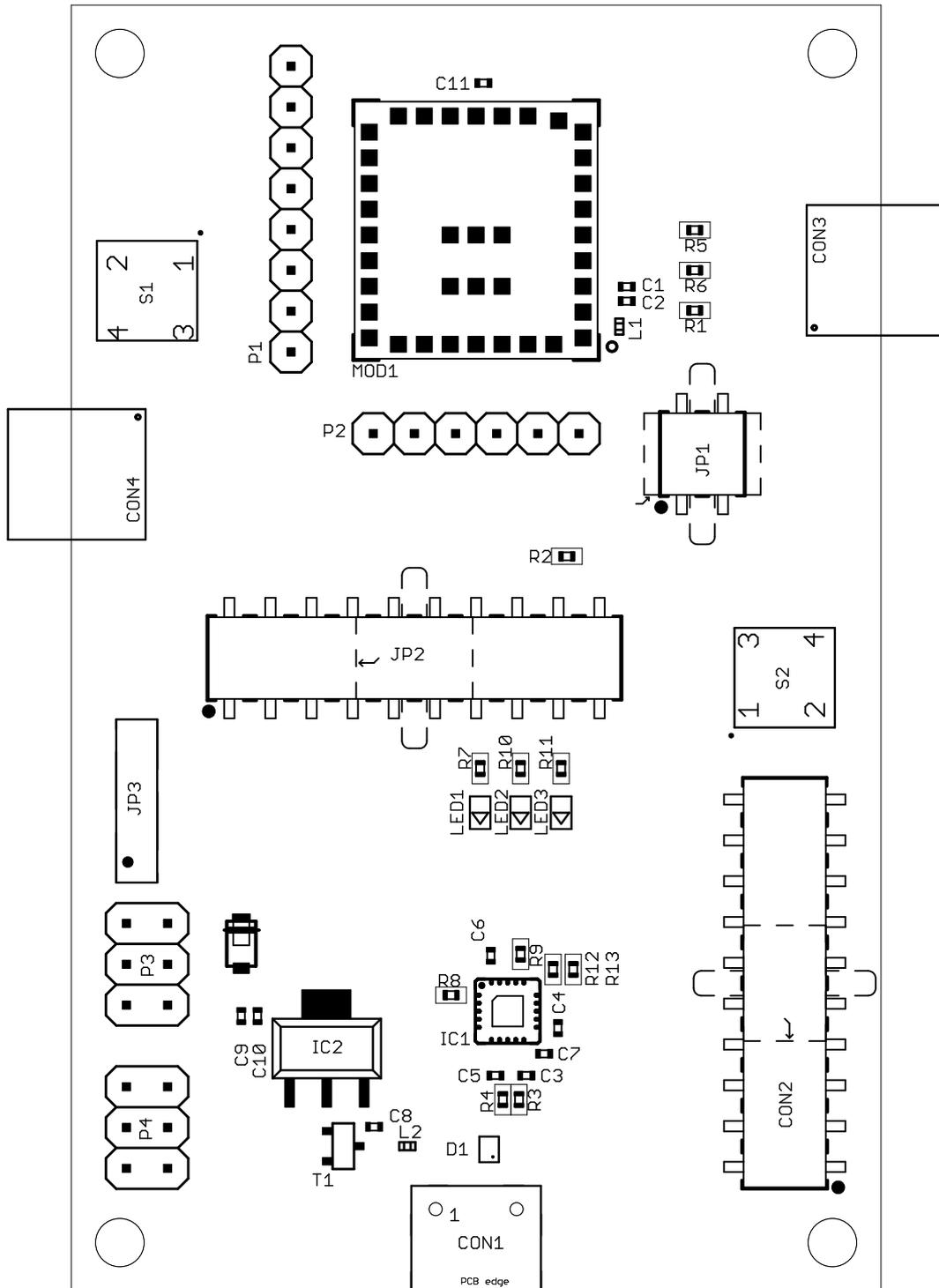
Figure 51: Reference design: Assembly diagram
