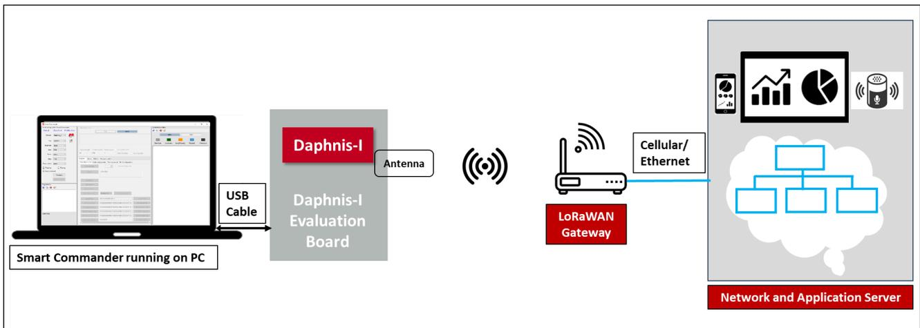
Figure 7: Daphnis-I quick start setup
